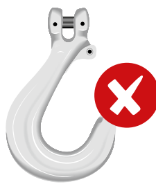
Don't use hooks without latch, as an exception is the foundry hook.
