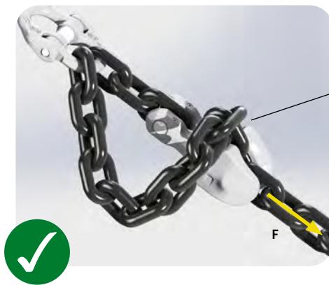
Load (F) bearing chain always needs to be at the bottom of the shortening clutch.
