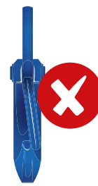
Hook body and latch may not be bent. This is a sign the hook is overloaded.
