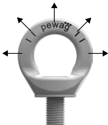
Permissible load directions
