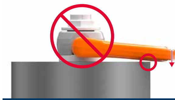
Improper loading as loading ring rests against edges or surfaces
