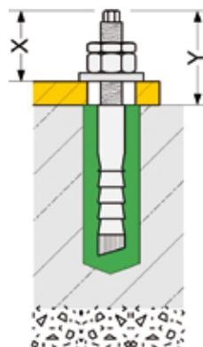
The smallest possible projection of the chemical anchor over the crane base plate "X" with an M12 anchor is approx. 33 mm, with M16 approx. 37 mm. This dimension can only be reached, if the concrete floor slab exceeds the above-mentioned min. thickness. The max. projection of the chemical anchor, measured
