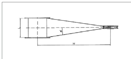
The distance between rope drum and sheave must be selected in a way that the maximum deflection angle for the type of rope used is not exceeded:
