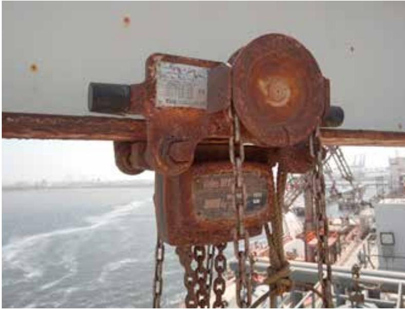
Corroded Yalelift with integrated trolley
