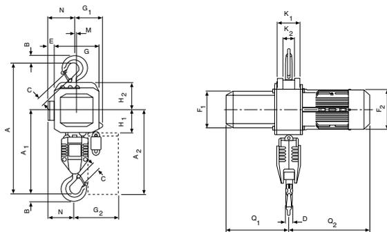
CPE<sup>1</sup>/CPEF with suspension hook, 3200 - 5000 kg, double fall
