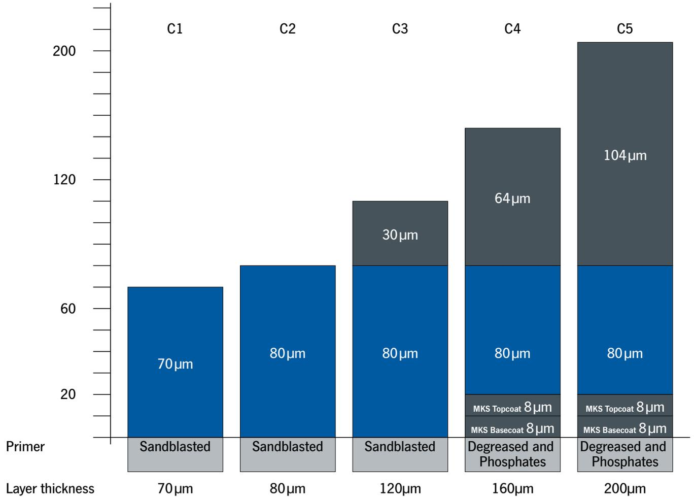
Up to C3 we cover all standard coatings (wet painting and powder coating) on our products. This means that the corrosivity categories C1 and C2 are also covered.
