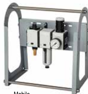
Mobile maintenance unit
