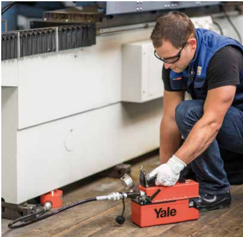
Ideal application in combination with compact, portable hydraulic tools like spreaders, lifting wedges, low profile and flat cylinders as well as nut splitters
