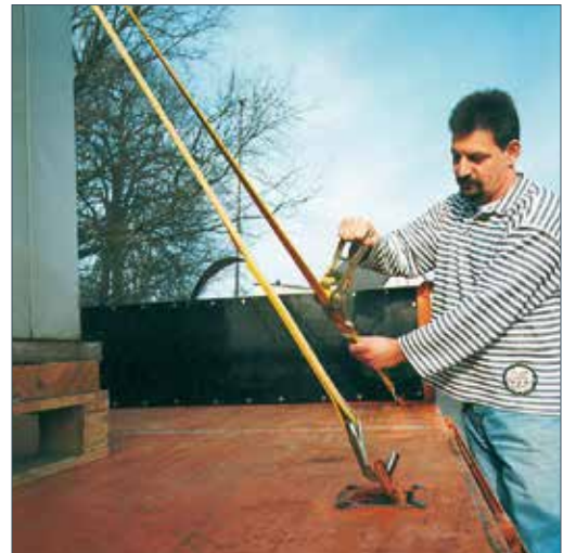
SPH - with double J hook
