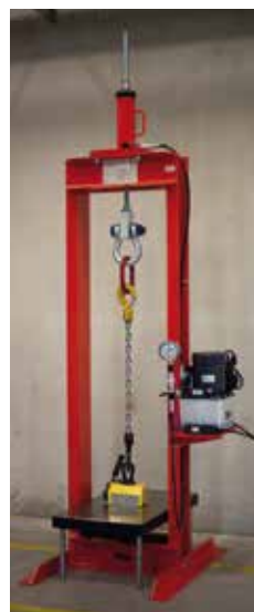
Permanent load lifting magnet TPM 0,3 for a test in the test rig RPYS-1215 complete with the test plate AYP-1215-S
